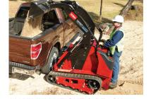
MAXIMUM HEIGHT & REACH 81" hinge pin height allows operator to dump into 30-yard dumpster or side of one-ton truck.
